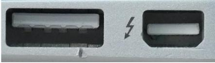
This is an almost square socket, with 2 cut-off corners. This is actually a Mini DisplayPort socket and Mini DisplayPort to HDMI adaptors are available at less than £20.
