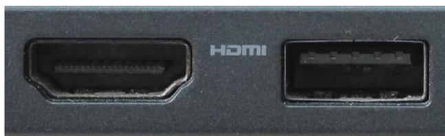
For comparison, on the right is a USB Type A socket, which is normally used for connecting peripherals like keyboards and mice. The HDMI socket is a little wider than the USB socket and it has two corners cut off at an angle. If you have an HDMI socket on your PC, all you need is an HDMI cable to connect your PC to your TV.
