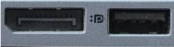
The DP socket is noticeably wider than the USB socket (shown on the right) and has only 1 corner cut-off at an angle. In this case you will need an adaptor (or “dongle”) to convert DisplayPort to HDMI. The conversion is pretty simple and so the adaptors are quite cheap, typically less than £10. DisplayPort to HDMI adapters are available from Amazon, Argos, PC World and many places on-line.
