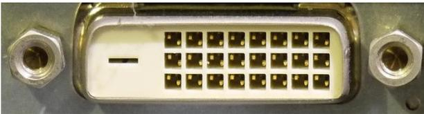
This was used on some older desktop PCs and laptops. DVI (Digital Video Interface) was a forerunner of HDMI and does not require signal conversion – you just need a DVI-HDMI cable, which is available at just under £20. Unfortunately, there is no audio connection in DVI, so you will need a separate audio connection to an audio system. DVI also lacks some of the automatic features of HDMI, so you might have to do some manual setting up on your PC.
